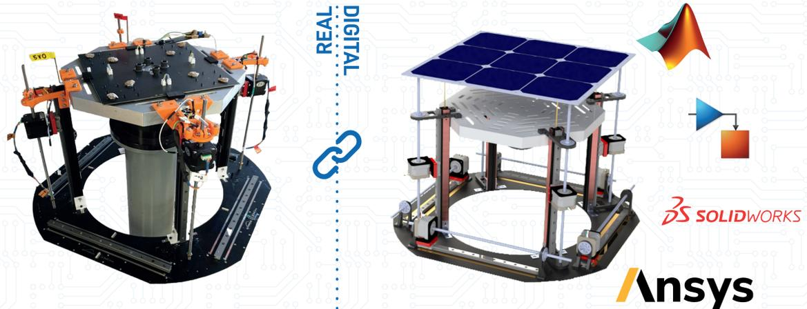
Figure 1: STASIS in development at PoliMI on the left; some of the engineering tools associated to its digital twin on the right
