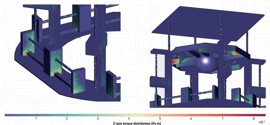
Figure 5: High pressure torque areas on STASIS identified through the CFD simulations
