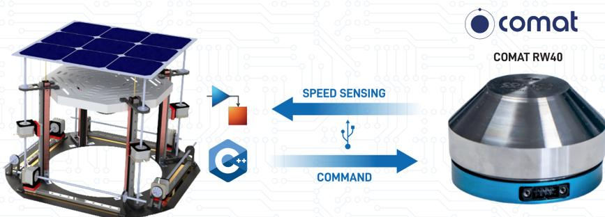
Figure 4: The digital twin of the platform was augmented with ready-to-deploy C++ code to be interfaced with the RW40 reaction wheel from COMAT. The speed data as read from the RW40 were fed back to the multi-physics simulation to investigate the performances of different attitude maneuvers
