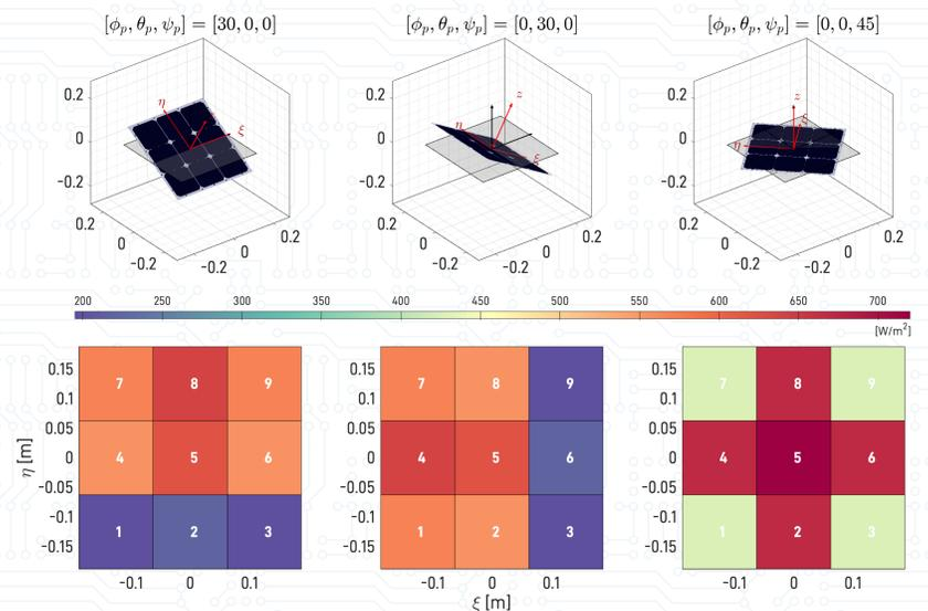
Figure 3: Beam irradiation distribution for different platform orientations, 9-cell configuration
