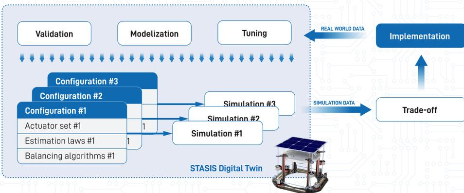
Figure 2: Design and simulation flow within the digital twin approach employed for STASIS
